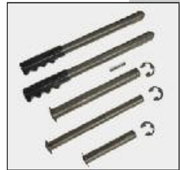
D54 Pin for D50 Locking Dog D55 Pin for D51 Heel Block D56 Pin for D53 Idle Pulley D57 Pin for D52 Floating Pulley (All Pins 1" Diameter 4140 Heat-Treated Alloy Steel).
